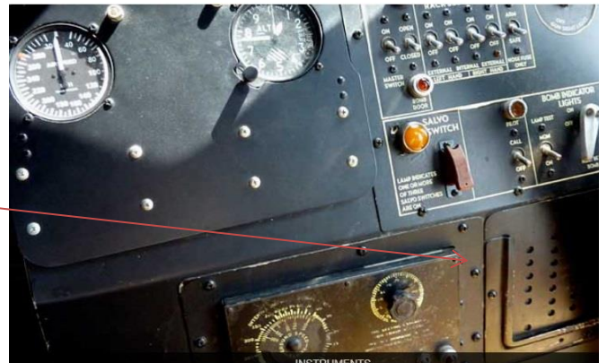
Figure 36-5, Bombardier station with the bomb load indicator. Zone-3. web. WWIIBRPG
