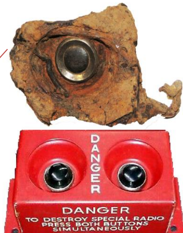
Figure 45-2, The BC-765 Switch Box is part of the SCR-595 Identification Friend or Foe (IFF) radio systems. In the event of potential capture of the aircraft by the enemy, the crew was to destroy the IFF system. Web,
