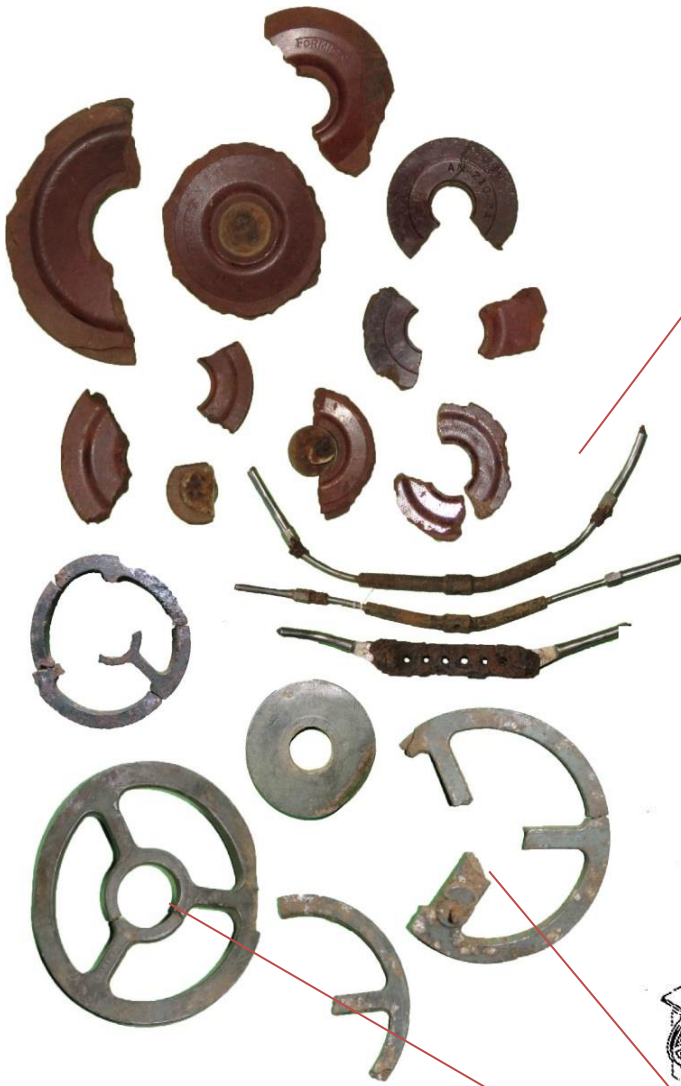
Figure 49-1, Throttle and Trim Tab controls, located in the center control stand, between the Pilot and Co-pilot. The pulleys here differ from the cable pulleys above and are made of aluminum instead of pressed Formica board. Also shown are a few cable connection joints, as shown in figure 49-2. WWIIBRPG, AN 01-20EG-4, web
