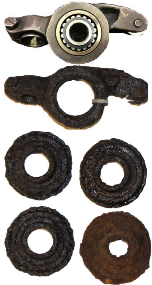
Figure 42-2, Internal engine parts found, here are some upper valve spring washers (PN 69271) and the Exhaust Rocker Arm (PN B9609), the latter compared to a new rocker
