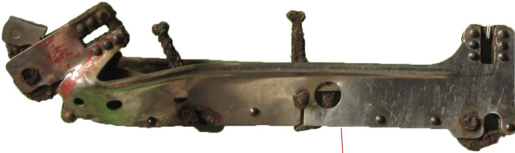
Figure 36-1, Bomb shackle Type B7, 100 – 1100 pound bombs, WWIIBRPG
