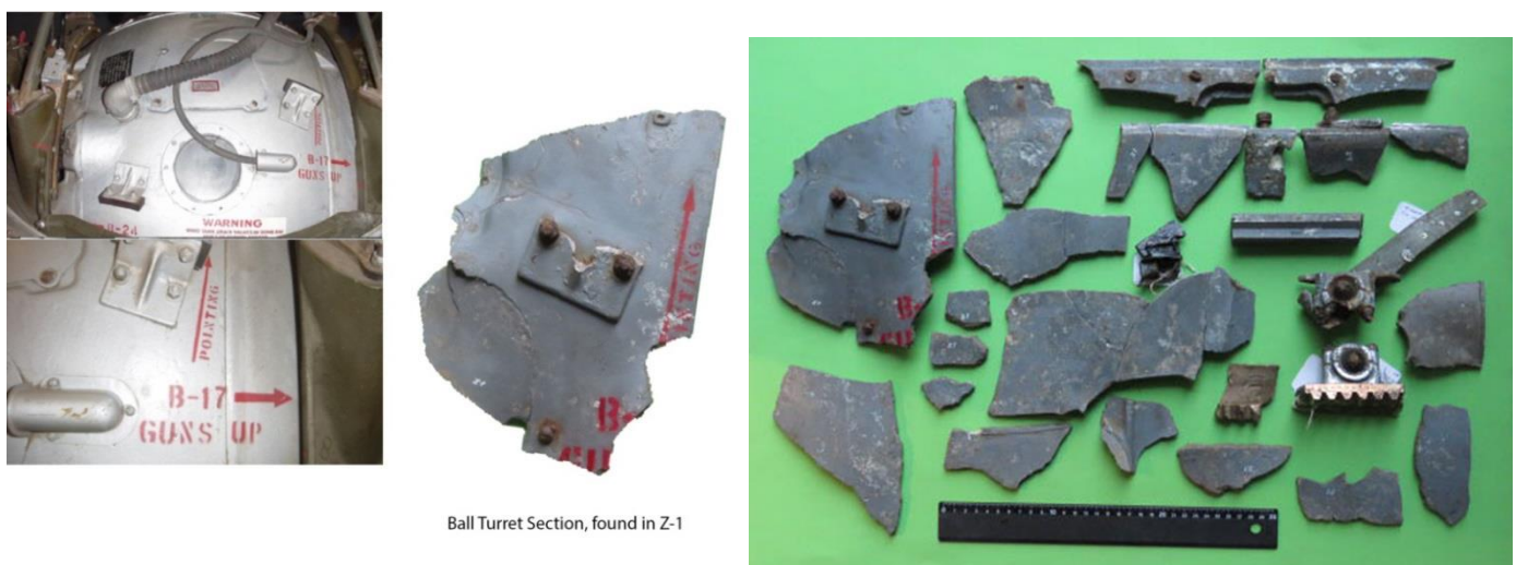
Figure 34- 2, Ball Turret Type A-2B or A-13A and fragments found, Web, WWIIBRPG
