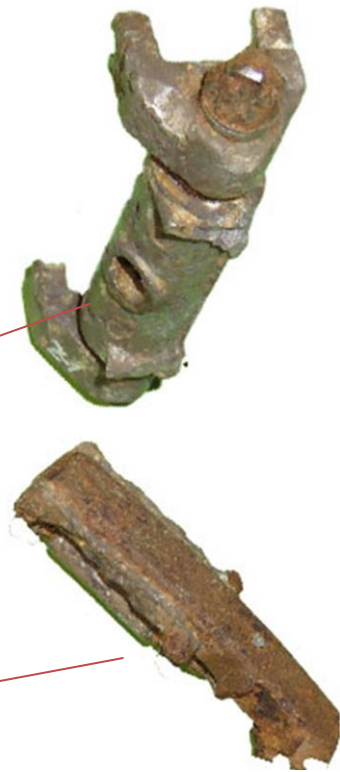
Figure 40-2 is another composite made of the piston chamber, sparkplug, ignition wire, and intake.
