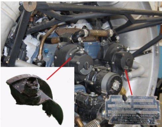
Figure 38- 3-4-5, Components of the engine include pieces of the Magneto, each engine had a left and right. The left magneto controls the firing of the rear spark plugs and the right controlling the front plugs. Web, WWIIBRPG
