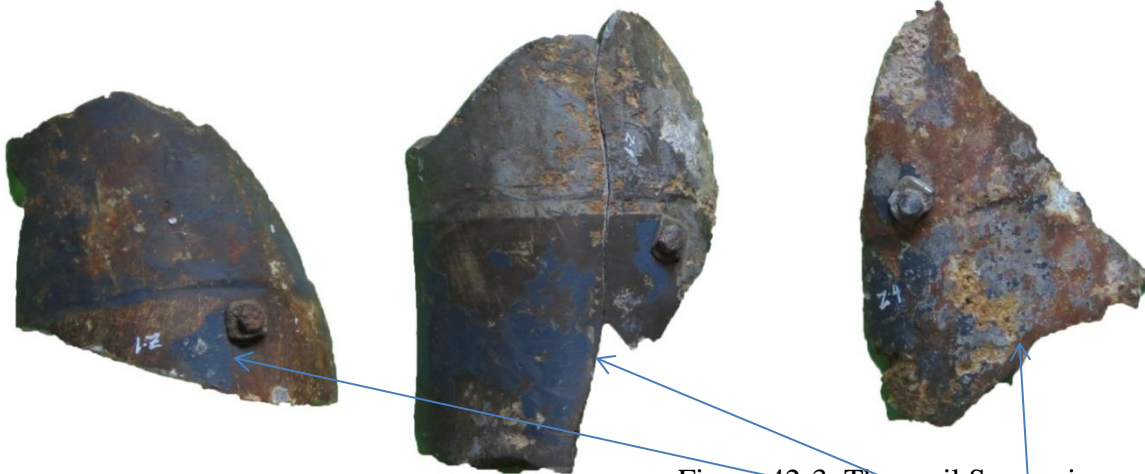
Figure 42-3, Three oil Sump pieces. This represents three different engines. Here in the squared area of the blue field is where the engine data plate attached. The complete sump is seen in Fig 39-2. WWIIBRPG
